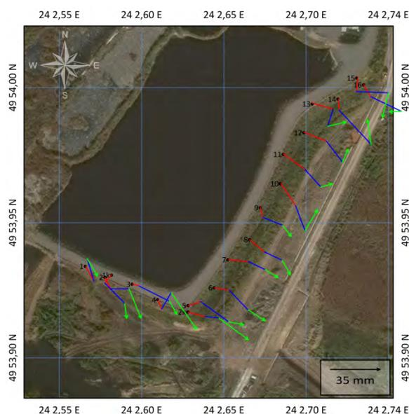
**Figure 2.** Scheme of the horizontal movements of the points (→ - between II and I cycles; → - between III and II cycles; → - between IV and III cycles)
