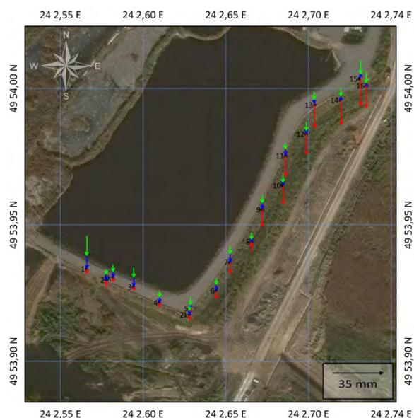
**Figure 3.** Scheme of the vertical movements of the points (→ - between II and I cycles; → - between III and II cycles; → - between IV and III cycles)
