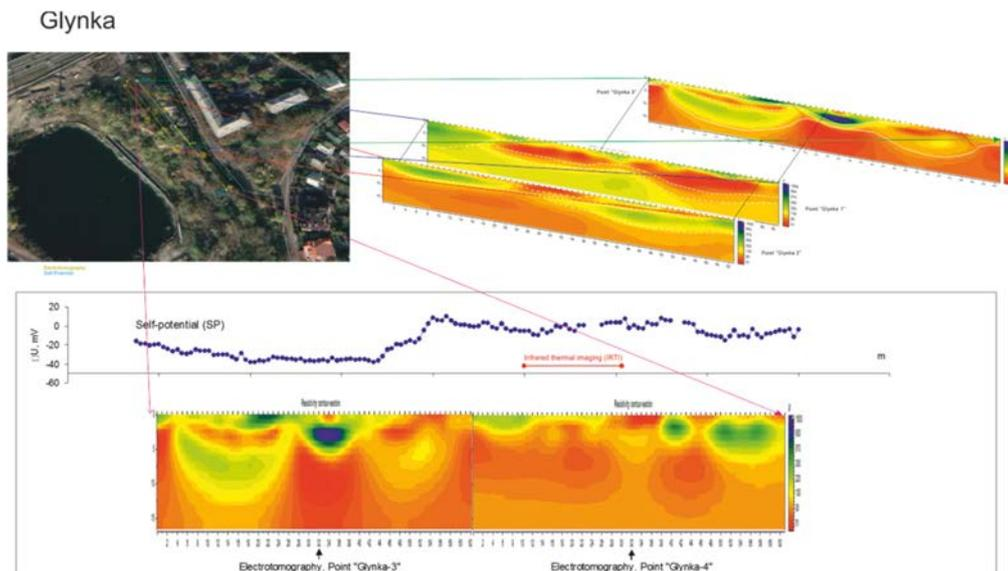
**Figure 3** Intergrated Self-potential (SP) and resistivity data, Glynka site
