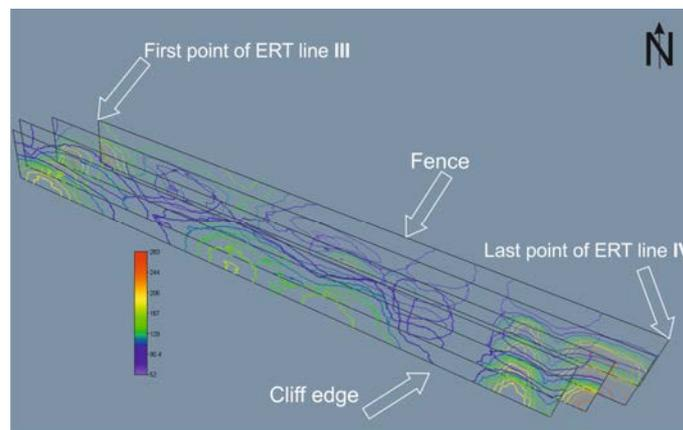
**Figure 4** Electrical Resistivity tomogram
