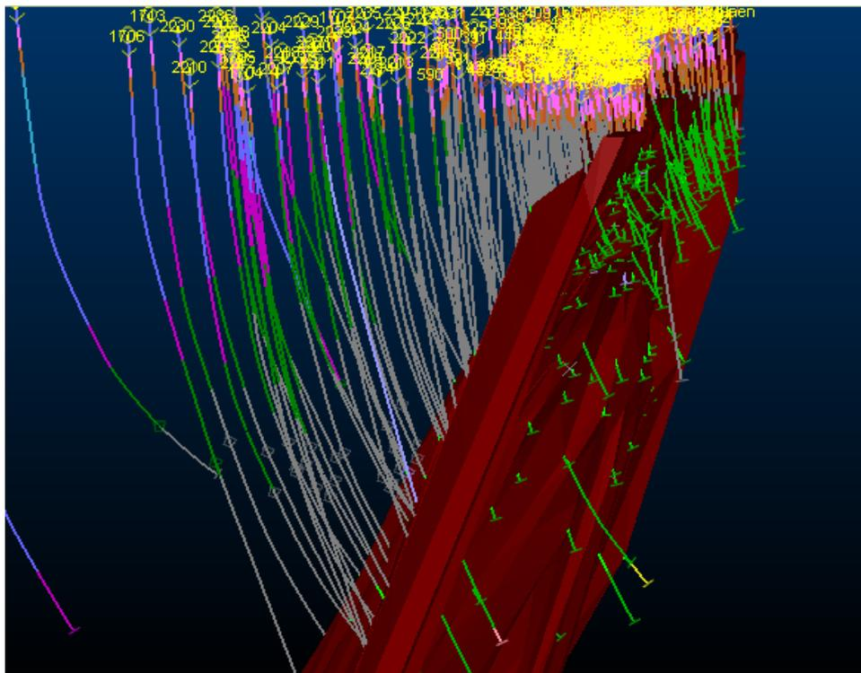
**Figure 3:** A wireframe model of the  $K_2^2$  ore deposit, which is crossed by boreholes.
