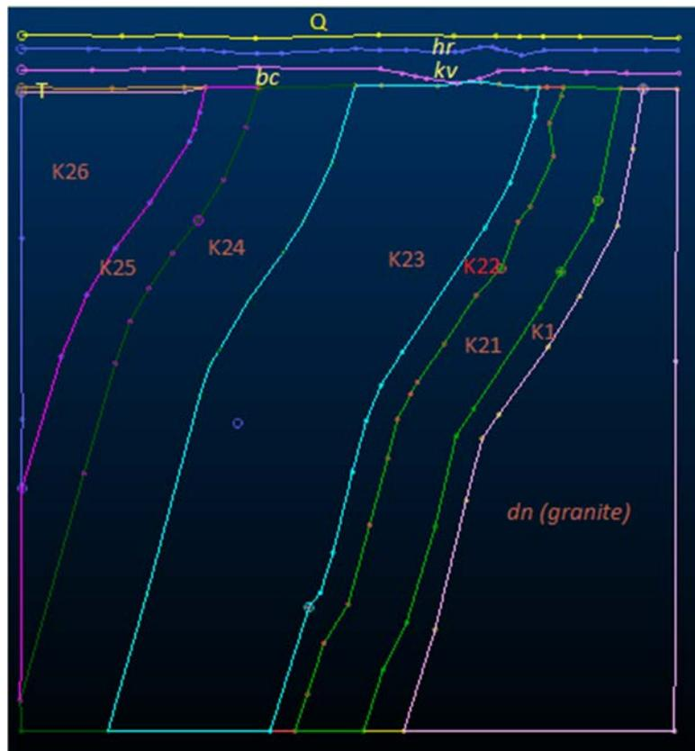
**Figure 2:** A geological section (profile XII). Note:  $K_2^2$  – ore pack, one last one ( $K_1, K_2^3, K_2^4, K_2^5, K_2^6$ ) – waste packs (Kryvyi Rych series); dn – Archean Dnieper complex granites; Q – quaternary sediments; hr – Kharkivska suite; kv – Kyivska suite; bc – Buchak suite; T – trias sediments.
