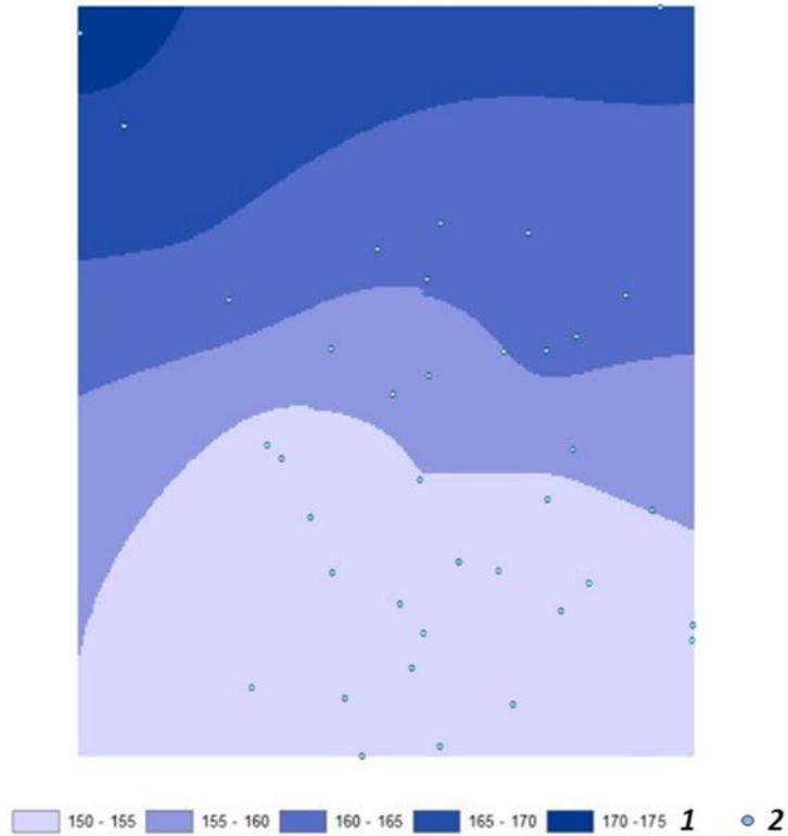
**Figure 1** The raster map of the field of layers of groundwater. 1 – layers of groundwater; 2 - wells
