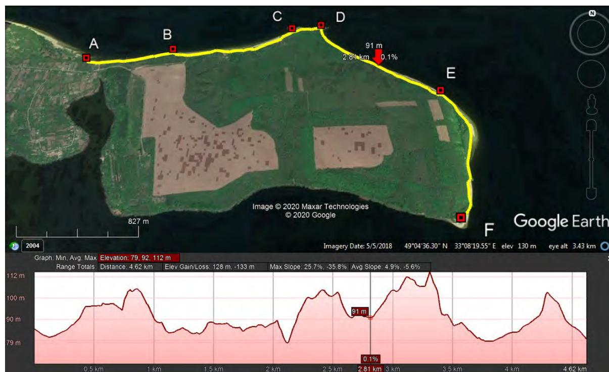
**Figure 2** Hypsometry of coast of the Kremenchuk reservoir within the peninsula Moscow Mountain (Google Earth Pro image): yellow line – hypsometry route; A, B, C, D, E, F – points of the route; horizontal and vertical scales – on the left side of the image; image orientation – to the north
