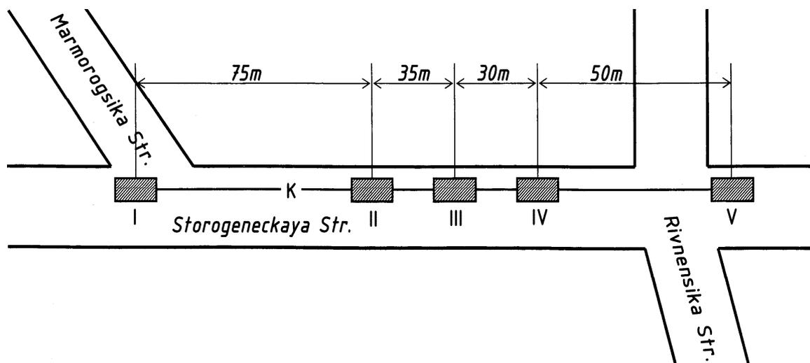
*Figure 1 Sewage pipelaying scheme*
