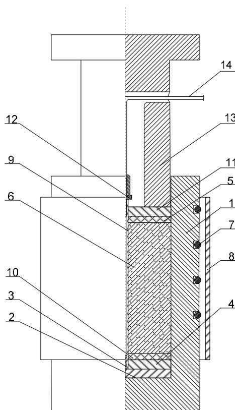
**Figure 1** Scheme of a high-pressure chamber for studying stress state of rocks: 1 – thick-walled cylinder; 2 – cylinder bottom; 3 – plug; 4,11 – steel washers; 5,10 – rubber gaskets; 6 – sample of the rock; 7 – heating element; 8 – protecting cover; 9 – steel pipe; 12 – adapter; 13 – plunger; 14 – inlet pipe
