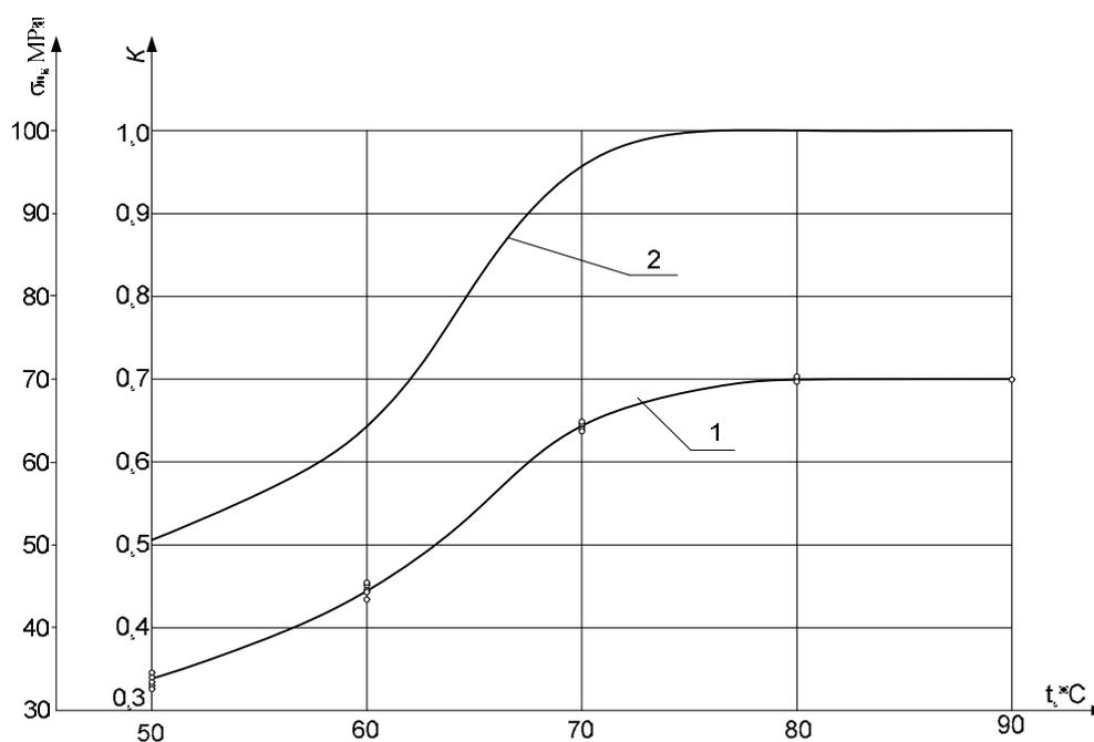
**Figure 2** Dependence of the lateral expansion coefficient of salt-bearing rocks (halite) on temperature ( $\sigma_z = 70\text{MPa}$ ): 1 – radial stresses ( $\sigma_r$ ); 2 – lateral expansion coefficient ( $K = \sigma_r / \sigma_z$ )
