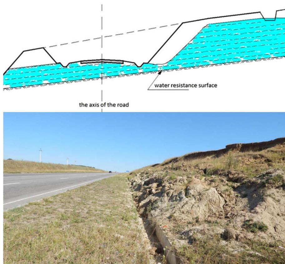
**Figure 3** Activation of landslide processes on the highway in Ternopil region. Sketch of the highway and photo of landslide by D. Pavlyuk
