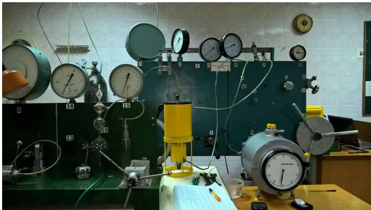
**Figure 1** General view of the working model of the UP-1 installation for determining the permeability coefficient of concrete, consolidated construction materials and rocks (stress-free and in tensile conditions)
