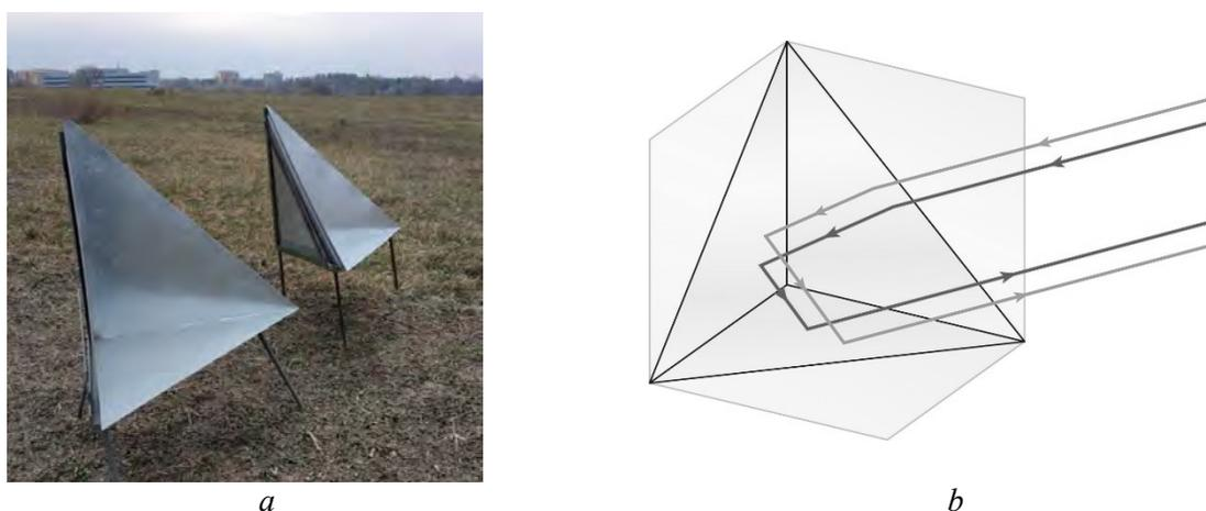
**Figure 1** a - Experimental corner reflector; b -The signal path through a triangular corner reflector
