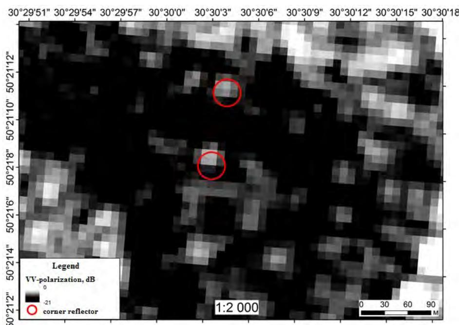
**Figure 2** Location of corner reflectors in the test region "Pirogovo" from 15.05.2019 against the background of satellite radar image Sentinel-1 (VV-polarization)
