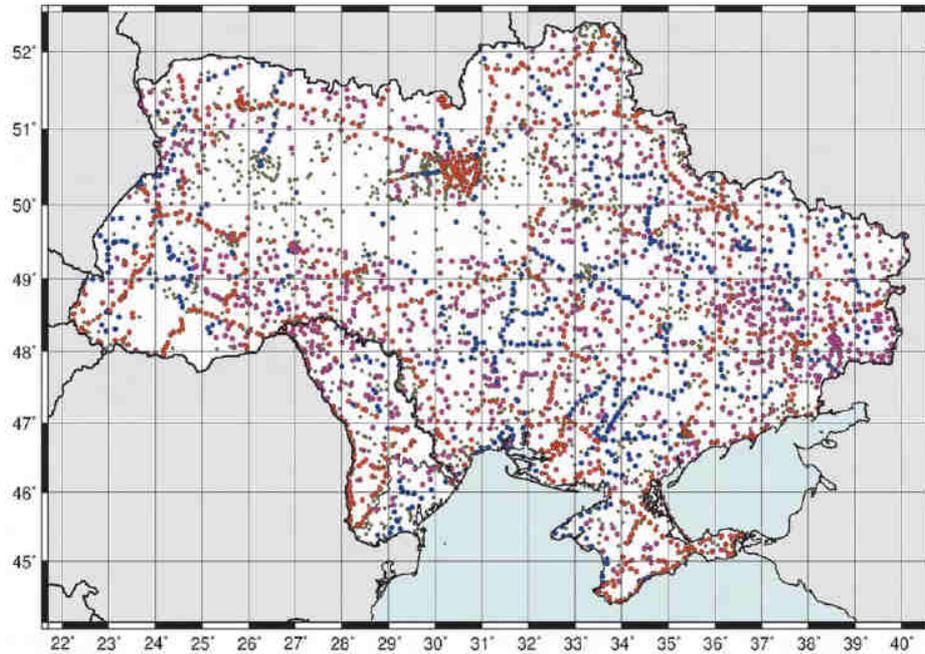
**Figure 1.** Distribution of GPS-leveling points of I (●), II (●), III (●) and IV (●) classes (Kucher et al., 2012)
