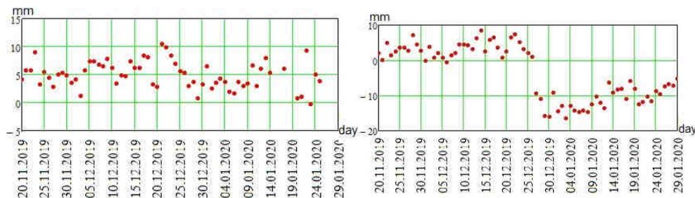
**Fig. 1.** A number of daily solutions of height deviation of GNSS stations of Geoterrace network in December 2019 (SULP – left, VYNO – right)
