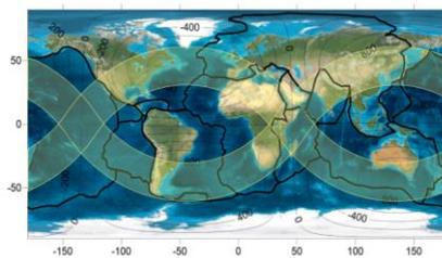
**Figure 4.** Maps of the distances between ellipsoids approximating the surface of the lithosphere and the geoid of the Earth
