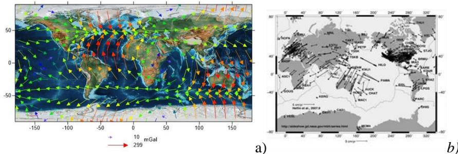
**Figure 3.** a – Maps of tangential forces versus the background of continents and oceans. The arrows indicate the tangential forces in milligals., b –. Map of horizontal displacement vectors of permanent GNSS stations (<https://i.ytimg.com/vi/KxJXiV4oTx0/maxresdefault.jpg>)
