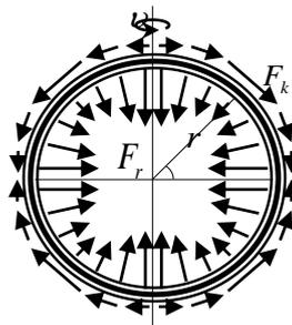
Figure 2. Illustration to the definition of forces  $F_r$  i  $F_k$
