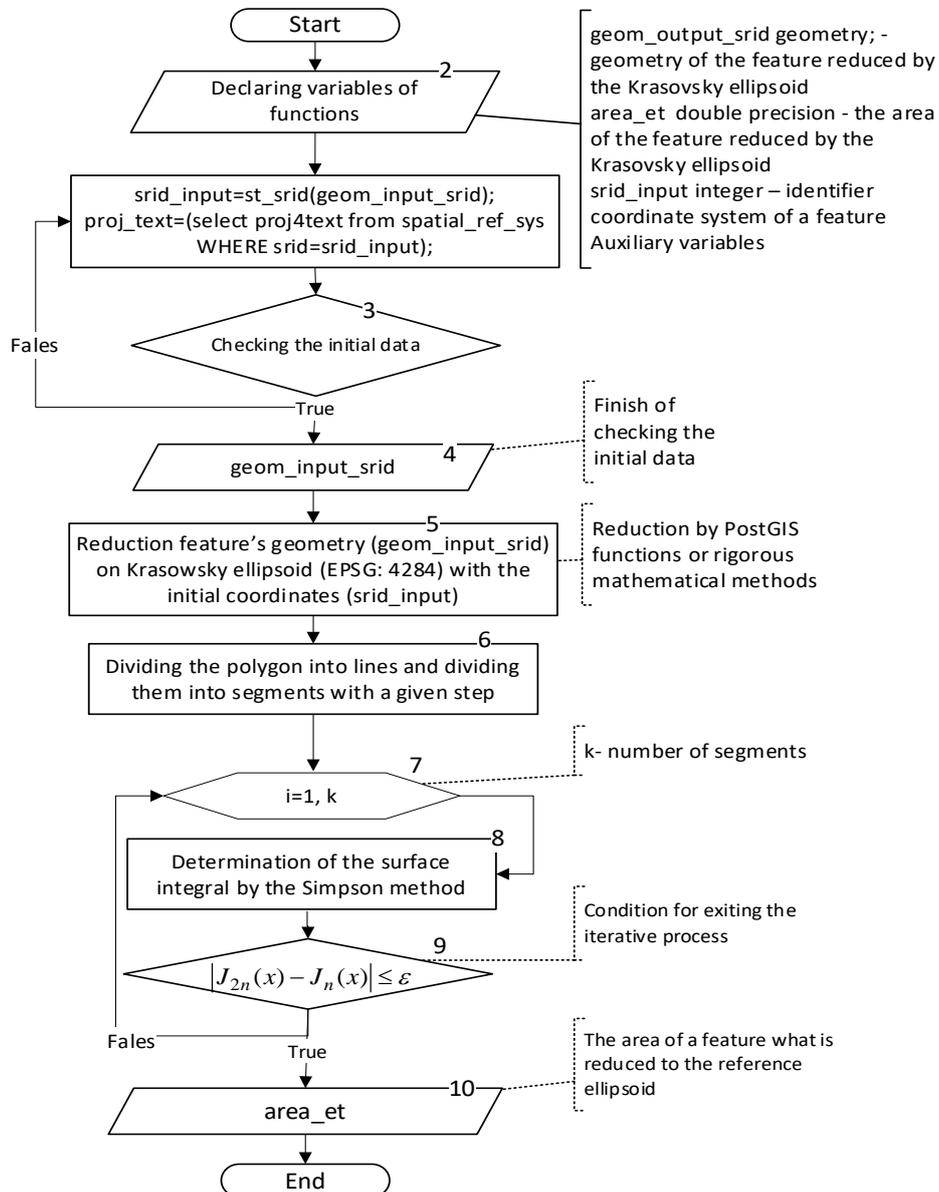
**Figure 2** The block diagram of the method of calculating the geodetic area on the ellipsoid by the method of the approximate contour integration
