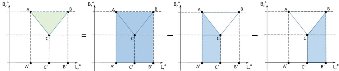
**Figure 1** Scheme for the calculation the area of a feature as an algebraic sum area of curvilinear trapezoids
