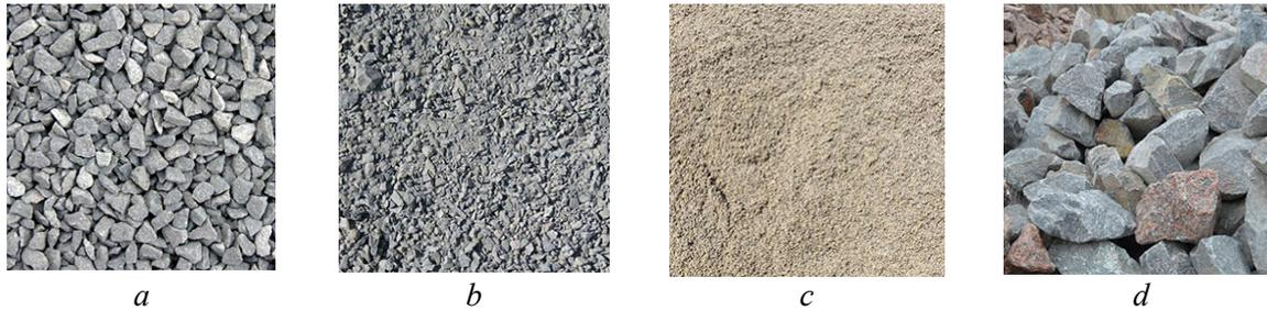
**Figure 3** Products of Boguslavsky Granite Limited Liability Company: a - crushed stone; b - gravel-sand-mixture; c - sand from crushing screenings; d - rubble stone (<http://www.bgkcomspec.com.ua/>)
