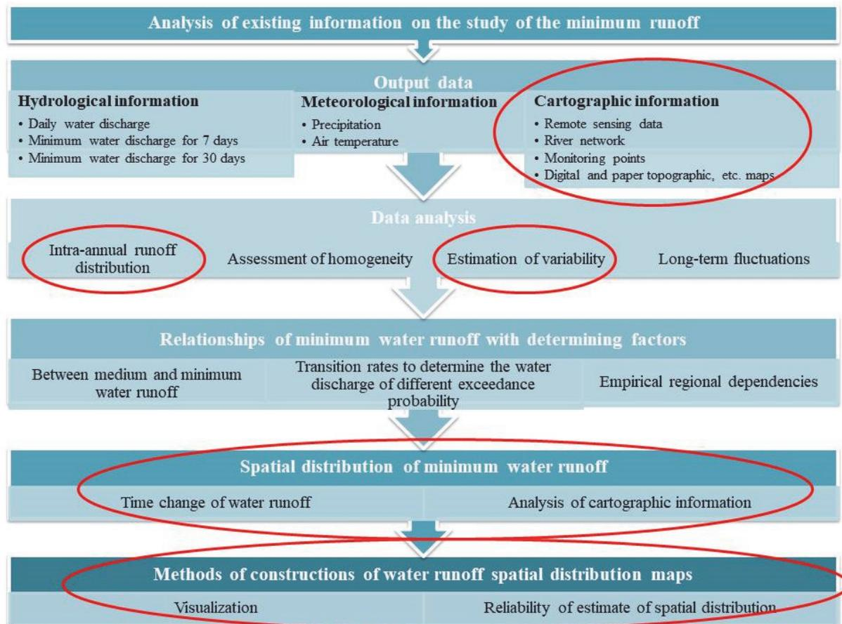
**Figure 1** Algorithm for estimating the minimum water runoff of mountain rivers
