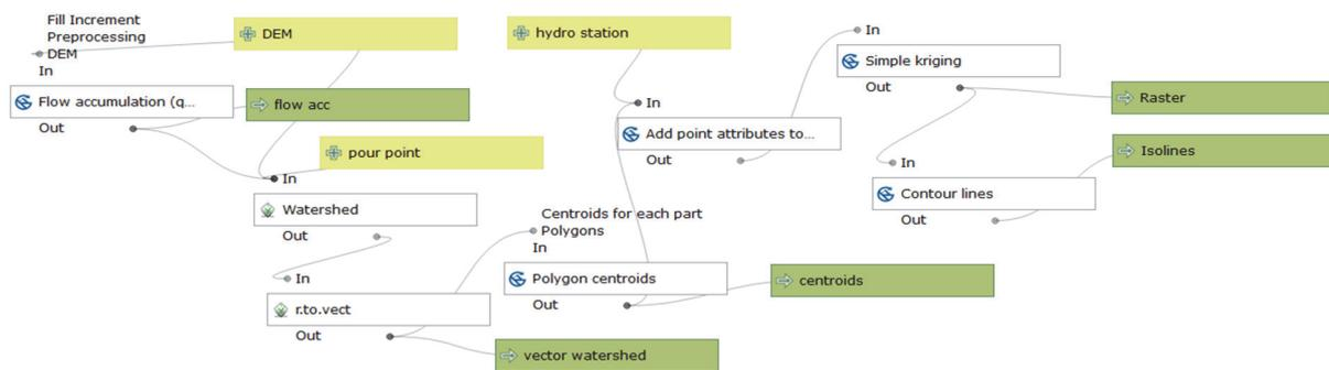
**Figure 2** Algorithm for constructing a map of modules of minimum water runoff in QGIS
