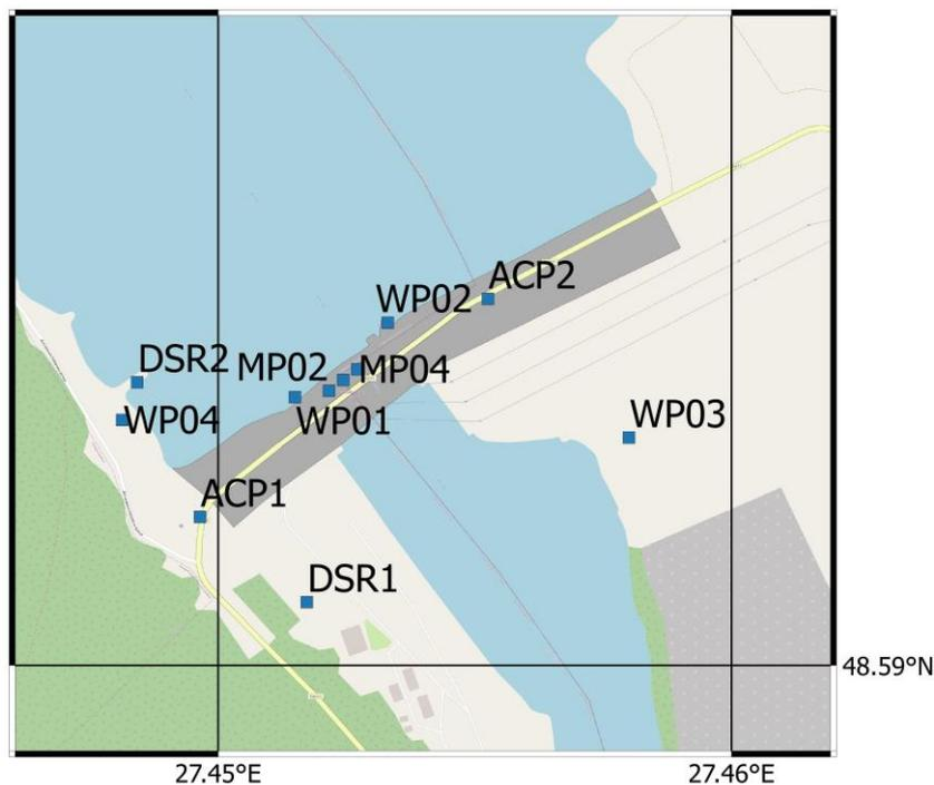
**Figure 2** Location of permanent GNSS stations of Dnister HPP-1
