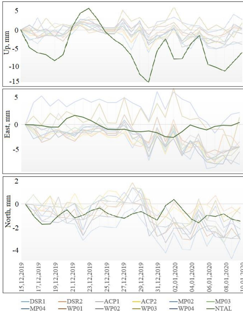
**Figure 3** Time series of up, east, north position changes of GNSS stations of Dnister HPP and modeled NTAL loading during the short-term subsidence in Europe (Brusak & Tretyak, 2020)
