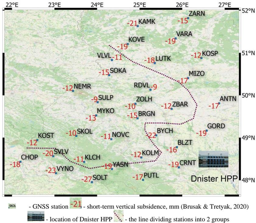
**Figure 1** Analysis of the dynamics of vertical displacements of GeoTerrace network in December 2019
