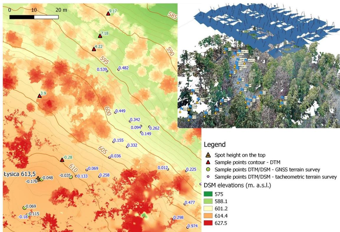
**Figure 2** The set of sampling points on the area of photogrammetrical flight. Residuals of DSM – terrain survey indicated in meters. Contours generated of the ALS - derived DTM. Sketch of the flight and point cloud in upper right corner of the figure.
