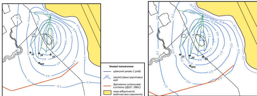
**Figure 4** Maps-schemes of groundwater level decrease in comparison with inverse problem at work of designed drainage located on 1m (above) and 2 m (below) groundwater level.
