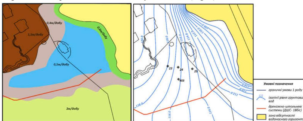
**Figure 3** Hydroisogypsum (absolute marks of groundwater level) according to the solution of the inverse problem.
