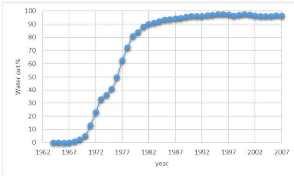
**Figure 1** The graph of the Water cut in extracted fluid at Lelyakivske field.
