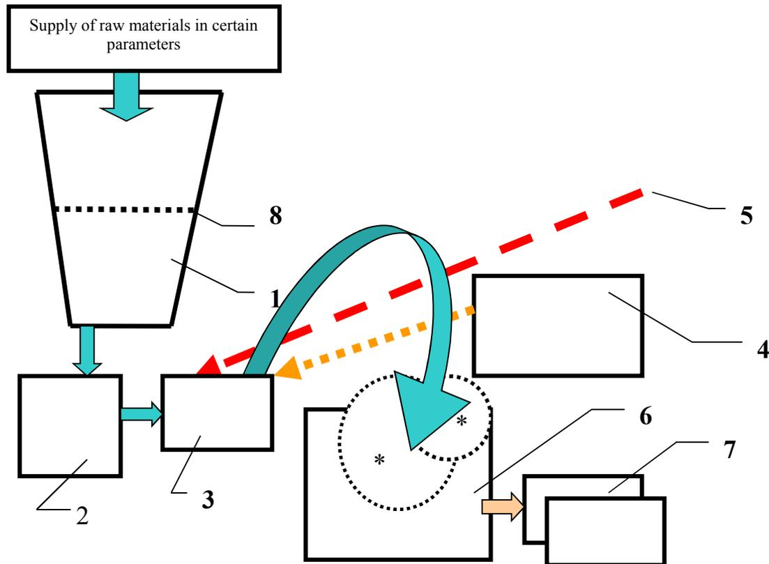
*Designation: 1 - bunker; 2- chopper; 3- mixer; 4- container for gluing elements; 5- container for a specially designed emulsion; 6- rotary press (operating in certain modes and technologies); 7- installation for briquetting a metal package. 8-mechanical sieve.*
