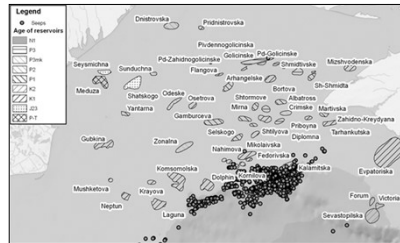
Figure 1. Comparison of main reservoirs of oil and gas deposit structures with areas of gas seeps (according to S.V. Goshovskyi)
