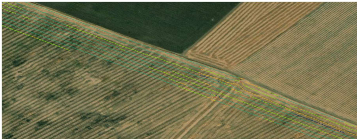
Figure. 2. Fragment of grain harvester movement trajectories based on GNSS monitoring data
