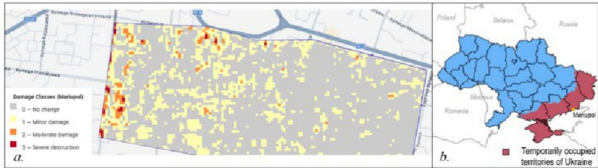
Figure 1. a. Result of damage classification based on Sentinel-2 Surface Reflectance data. b. Study area. The map shows temporarily occupied territories in red (KMZmap, 2026; Free Map Tools, n.d.)
